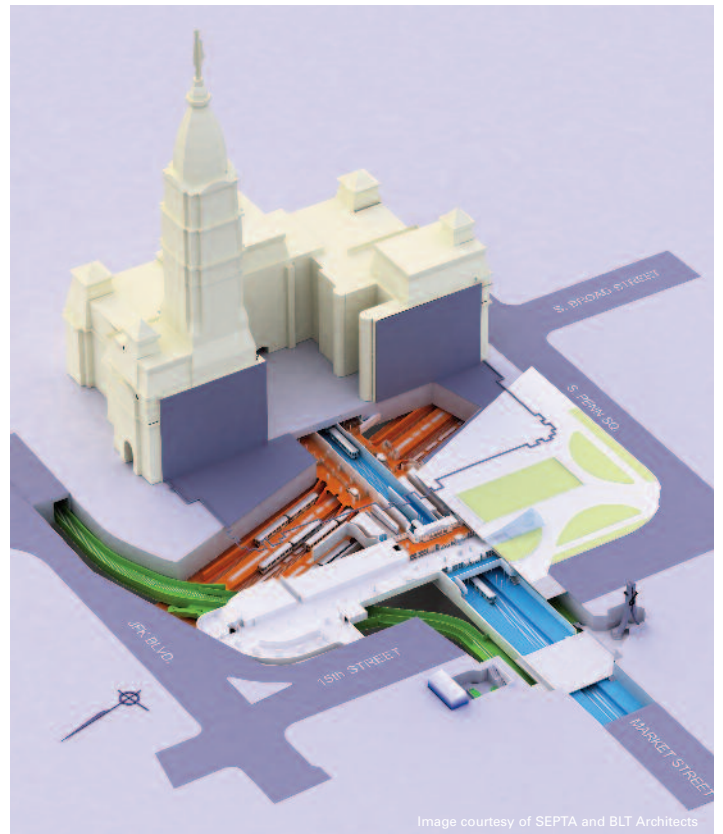
A cross-section reveals the multiple levels of transit infrastructure beneath City Hall and Dilworth Plaza.
